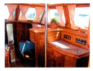
The enclosed pilothouse features large thermo-pane with low E-coating and light grey-tinted windows forward and outboard, and aft is a custom retractable window with screen to the cockpit. There are four-opening rooftop hatches.
