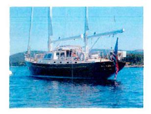
Hydraulic stoway, three-spreader cutter/ketch rig.
